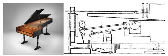
Above is a picture of the first piano and next to it is the diagram of its action. Some parts that you may be able to recognize are the key (K) and the hammer (A and B). The string is pictured at the top. The damper, though it is not labeled, is to the far left end of the string. At this link (https://youtube.com/watch?v=uZjcV3\_0PqQ), you can find a video of this "action" in action.
